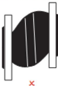
Out of Line Connections
