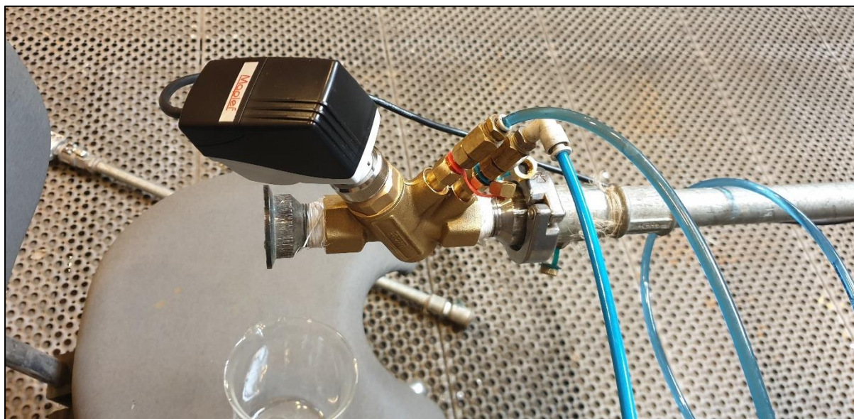
Figure 11 Seat leakage test setup
